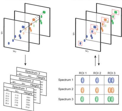
**Figure 1.** Traditional (A) *versus* ROI-based (B) analysis of two-dimensional NMR data. Traditional approaches for matching signals across multiple spectra are prone to error because of chemical shift variation. The ROI-based approach used by rNMR avoids this problem by allowing users to view all of the NMR data related to a resonance assignment, and to dynamically resize or move ROIs so that only the target signals are included in any analysis.
